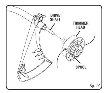
Hold the spool so that its tabbed side is positioned upward.
